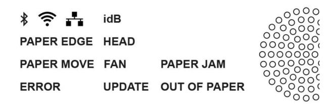
The backlight's top row consists of the Bluetooth icon, a Wi-Fi icon, and a wired network icon. Each of these light up when a connection of this type is established. The last item of the top row is idB, which stands for Index direct-Braille and lights up when Index's direct-Braille translation is in use.
